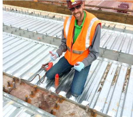
Figure 52 Magnetic particle testing and inspector
