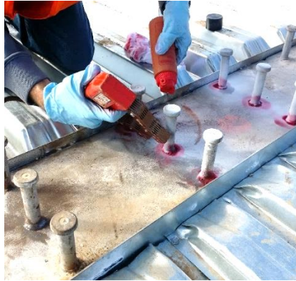
Figure 52 Magnetic particle testing and inspector
